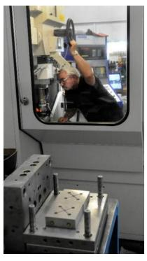
In this file photo, machinist Colin Saulnier sets up a CNC machine to drill holes in a steel mold cavity, like the one in the foreground, used to make plastic gears at ABA-PGT, Inc. in Manchester. The company began in 1944 as a machine shop making steel parts for Pratt and Whitney. (Bob MacDonnell/The Hartford Courant)
